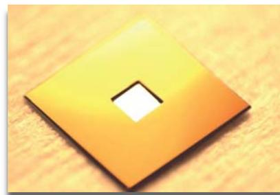
Top: SiN membrane used as the opto-mechanical resonator.
