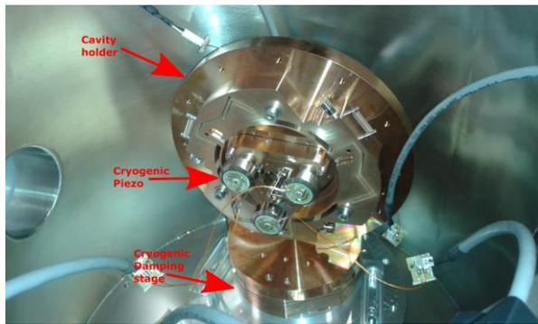
Figure: Photo of the optomechanical cavity. The arrows show the different components of the cavity. The cavity holder is mounted on top of a damping stage that isolates the optomechanical cavity from the cryostat. The cryogenic piezos are mounted on the mirrors of the cavity and allow to realign the cavity at cryogenic temperatures. The membrane is inside the cavity holder between the two mirrors.
