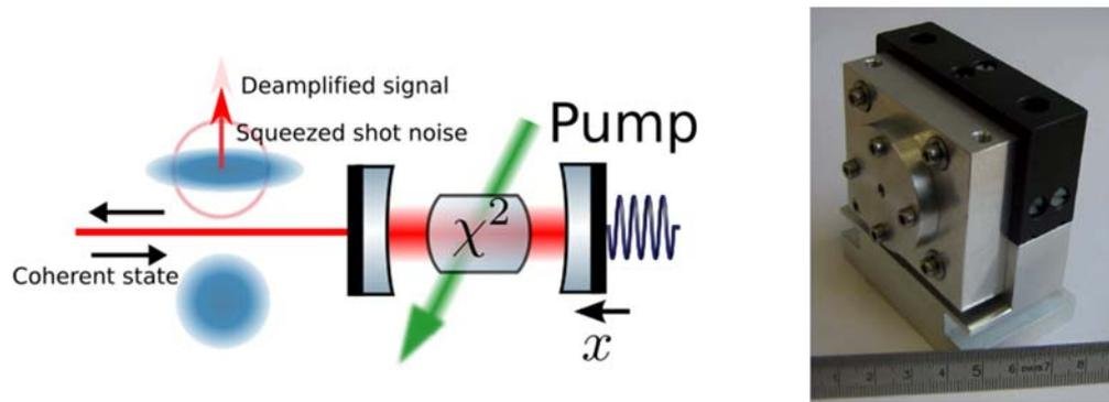
**Figure 1.** *Left:* the principle behind the internal squeezing: optomechanical interaction is amplified by the nonlinear crystal inside the cavity, the signal gets deamplified less than the shot noise squeezed, yielding gain in the signal-to-noise ratio. *Right:* optical parametrical amplifier cavity used in a proof-of-principle experiment on internal squeezing.
