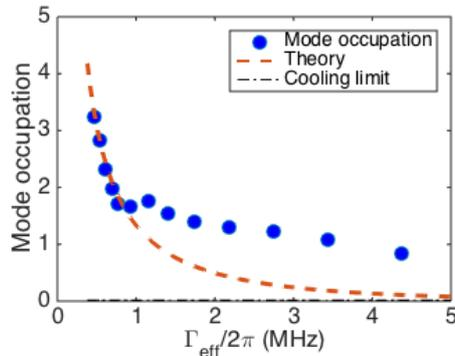
**Figure 2.** Mode occupation vs the effective damping rate of the mechanical oscillator through sideband cooling, in comparison to the theoretical mode occupation and sideband cooling limit.
