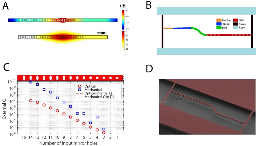
**Figure 1.** A) Simulated mechanical and optical field distribution, where the mechanical motion is perfectly confined while the optical field can be coupled in and out from one side of the cavity. B) Design of the device, which includes supporting pad, bridges, coupling waveguide, tapered waveguide, bended waveguide and one-sided photonic crystal. C) Simulations of the external optical Q and mechanical Q with different holes number for the input mirror. D) SEM picture of the actual device.
