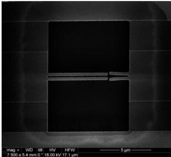
Figure 3: SEM image of cantilever mass sensor
