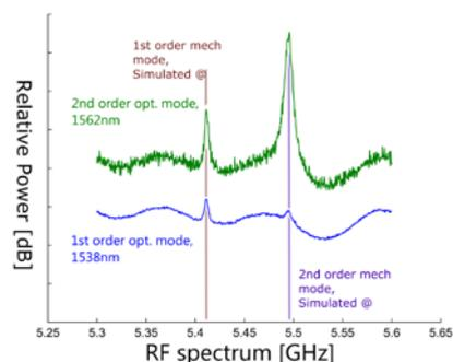
Figure 2: ESA measurement of the spontaneous vibrations in an optomechanical crystal.
