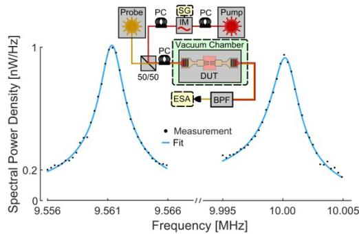
Figure 4: ESA measurement of stimulated vibrations in the mass sensor.
