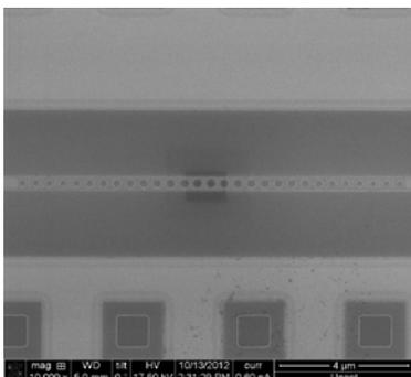
Figure 1: SEM of optomechanical crystal.
