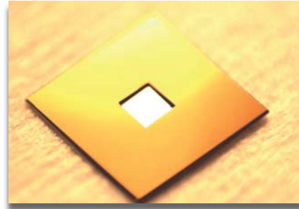
Top: commercially available SiN membrane used as the opto-mechanical resonator. Left: Schematic of the experimental setup. (shared work with Ramon Moghadas Nia)
