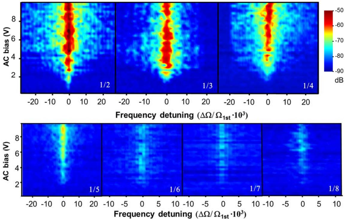
Figure 2: Superharmonic resonances of NOEMS platform for up to 8th order
