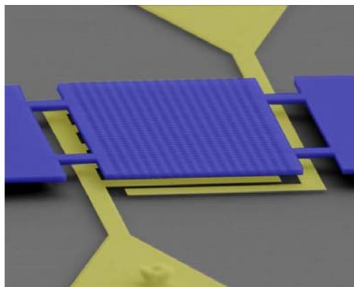
**Figure 1 : Suspended photonic crystal nanomechanical membrane over gold interdigitated electrodes**
