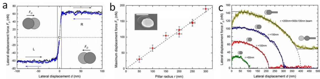
**Figure 2.** (a) Lateral displacement forces of 100nm radius and 60nm height graphite pillar. (b) Maximum lateral force of different pillar radii. (c) Full displacement force traces for both circular and combined circle beam structure.
