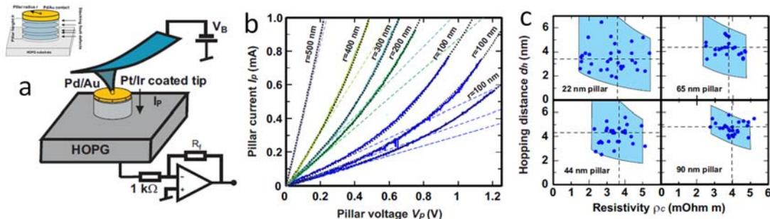
**Figure 1.** (a) Measurement setup, inset shows the presence of individual stacking faults along the c-axis. (b) i-V plots of graphite nanostructures of different radii. (c) Hopping distance vs. resistivity for different pillar height.
